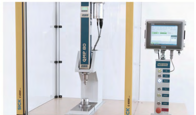
DSM press-fit station with protected working space for caulking of bushings.
